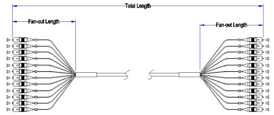
Pre-terminated Universal Cable System with Dual Staggered Fan-out
