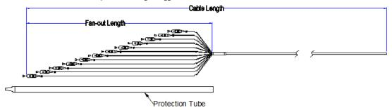
Pre-terminated Universal Cable System with Dual Fan-out
